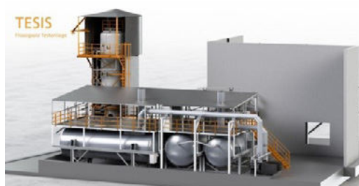
Abbildung 6 TESIS Test facility for Thermal Energy Storage (DLR)
